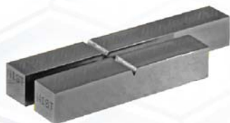
Figure 1. Examples of Charpy and Izod samples.
