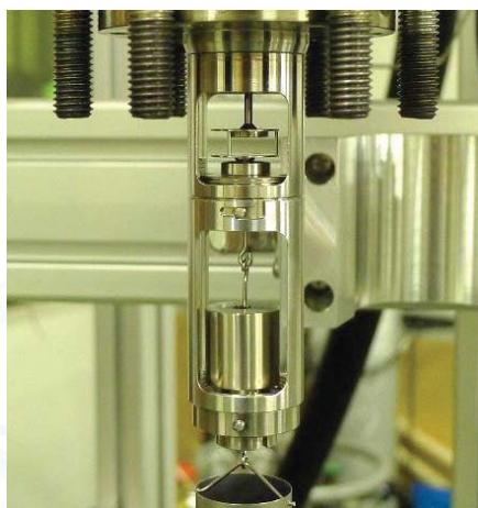
Figure 1. Combined tool for binary gases. A magnetic suspension balance monitors mass uptake without contact between the sample holder and measuring instrument.
