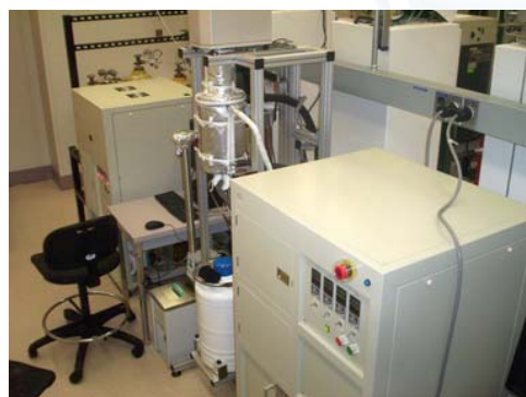
Figure 3. Combined Tools: Sorption isotherm measuring station for binary gas mixtures (bottom right) and volumetric tool with gas chromatography for multicomponent gases (upper left).
