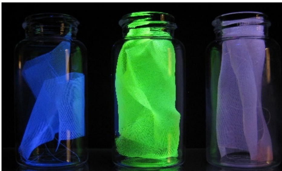
Examples of the silk used in experiments to detect damage in composites, shown under black light. (Left) Ordinary fibroin of the Bombyx mori silk worm. The observed fluorescence is the result of molecules already present in the protein structure of the fiber. (Middle) Mechanophore-labeled silk fiber fluoresces in response to damage or stress. (Right) Control sample without the mechanophore. Credit: Chelsea Davis and Jeremiah Woodcock/NIST
