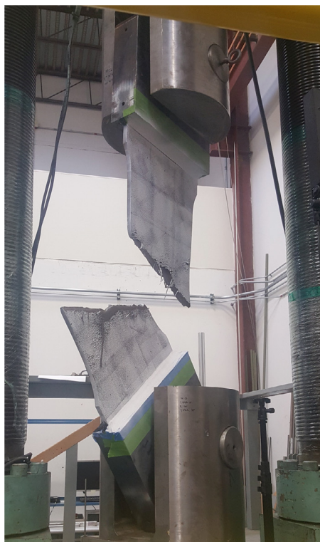
A sample of high-strength X70 steel pulled apart by NIST testing.
