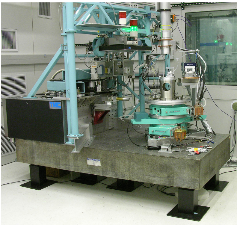
NIST's new X-ray machine for high-precision measurement of the Copper Alpha spectrum, shown here in its 0.01 degree Celsius temperature-regulated space. Credit: James Cline/NIST
