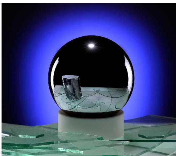
A nearly perfect 1-kg silicon sphere reflecting its connection with a 1-kg prototype platinum-iridium alloy cylinder. Credit: PTB
