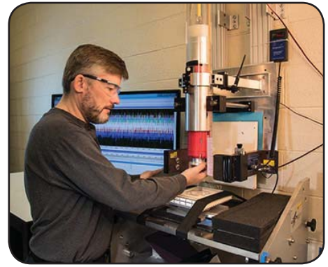
NIST MML materials scientist Michael Riley prepares a sample of material for a drop test that will reveal its ability to absorb and dissipate energy. This was one of a series of tests that helped the Head Health III judges identify five materials that held the most promise for bringing improvements to protective gear. Photo credit: Earl Zubkoff
