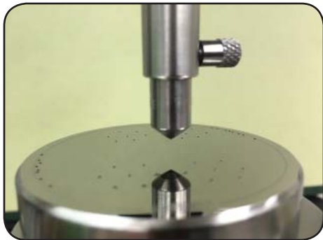
A Rockwell hardness diamond indenter positioned to make a test in the polished surface of a steel test-block standard.
