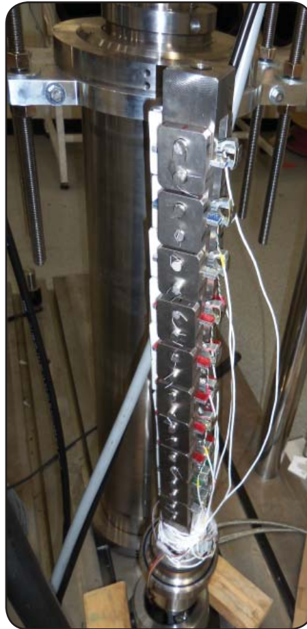
Samples of pipeline steel instrumented for fatigue testing in a pressurized hydrogen chamber (the vertical tube). NIST researchers used data from such tests to develop a model for hydrogen effects on pipeline lifetime, to support a federal effort to reduce overall costs of hydrogen fuel. Credit: NIST
