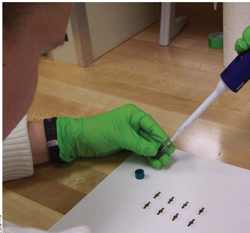
Small piezoelectric quartz crystals are the key to micro thermogravimetric analysis. Minute amounts of the test sample are deposited on the crystals.
