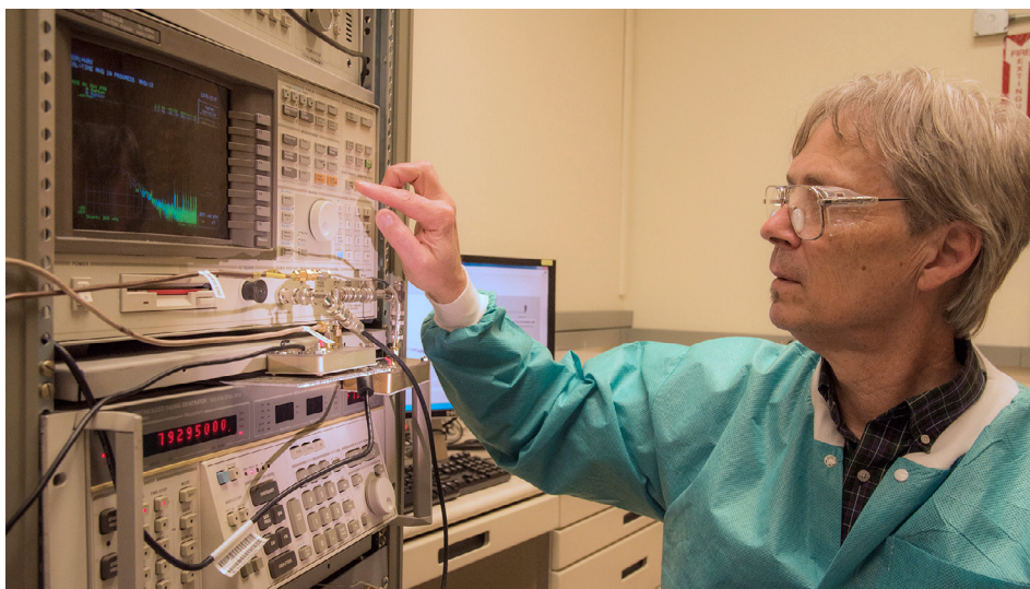
NIST physicist Ward Johnson observes signals generated by bacteria coating quartz crystals, a novel method of sensing whether an antibiotic kills the bacteria. The new NIST technique senses mechanical fluctuations of bacterial cells and any changes induced by an antibiotic. With further development, the technique could hasten the identification of effective medical treatments in clinical settings and drug development. Credit: J. Burrus/NIST
