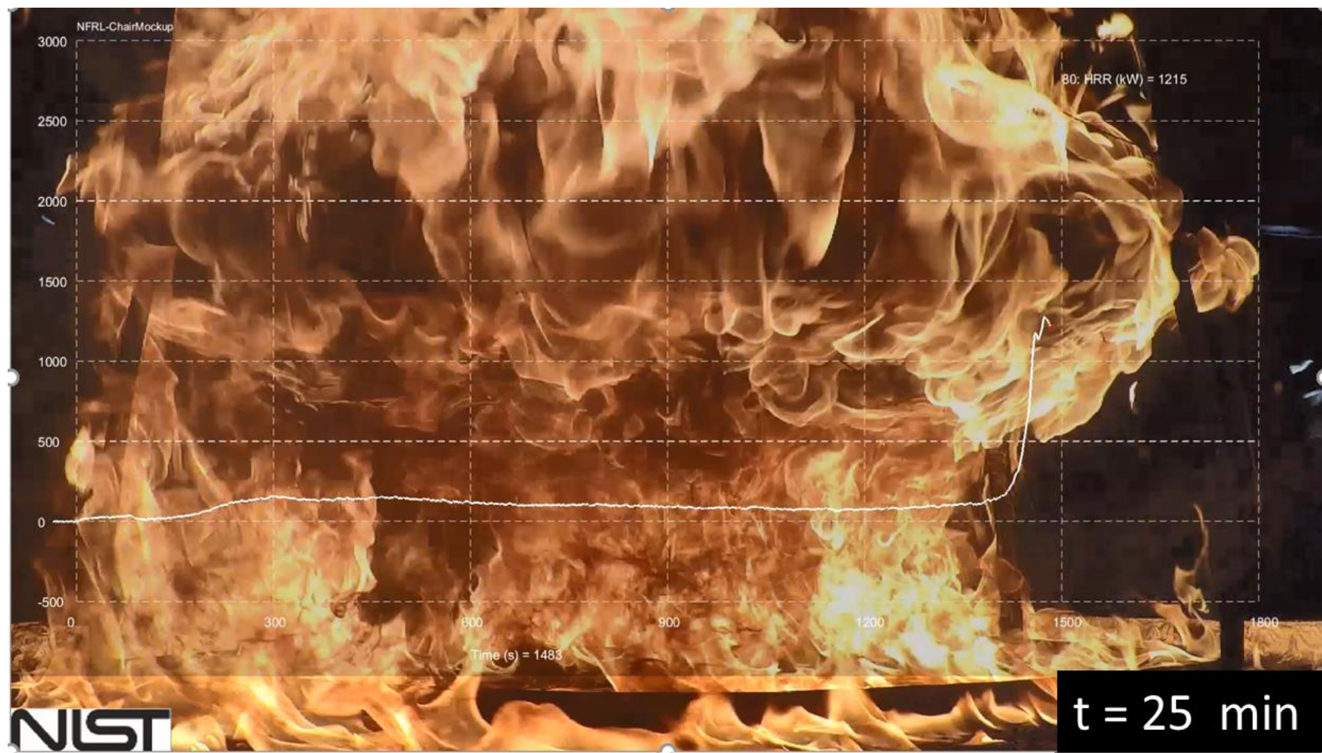
Bottom Ignition (BI): persistent burning under the seat cushion due to the ignition of liquid product of pyrolysis
