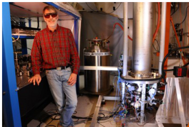
NIST-F2 laser-cooled fountain atomic frequency standard
