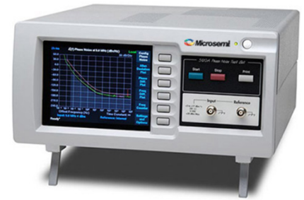
Microsemi digital phase noise metrology system
