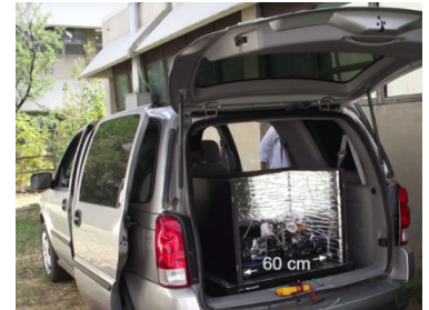
Miniaturized portable aluminum ion logic clock, operating in moving vehicle
