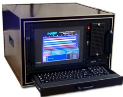
Remote time & frequency measurements in user’s lab. \Delta f/f \sim 2 \times 10^{-13} \Delta t \sim 1 \text{ ns}
