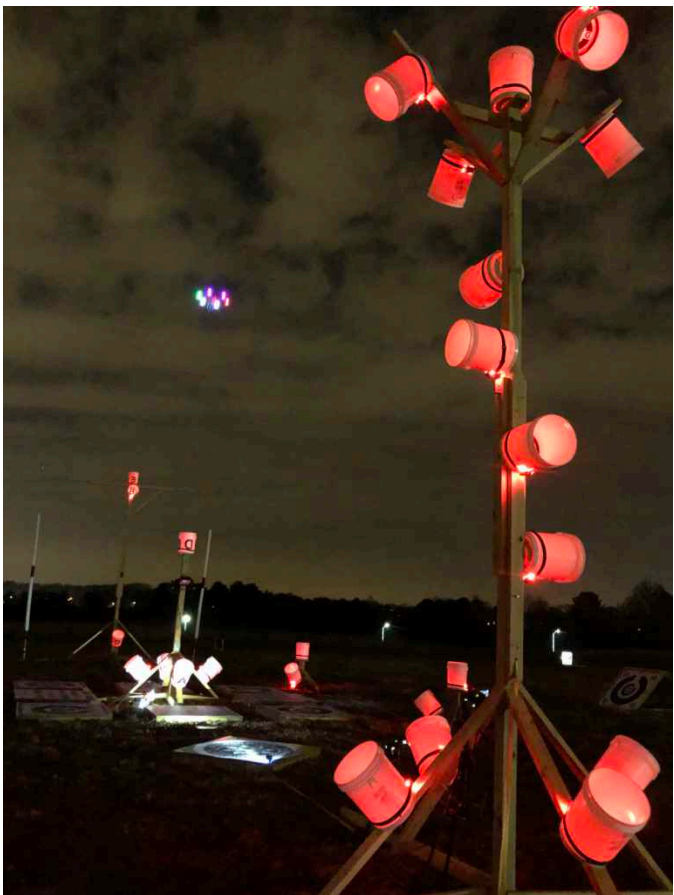
Position accuracy for range to target using lighted buckets (red or white)
