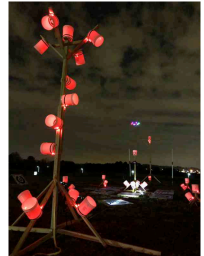
ILLUMINATED BUCKETS PROVIDE POSITIONING AIDS LIKE STRUCTURE WINDOWS OR STREET LIGHTS
