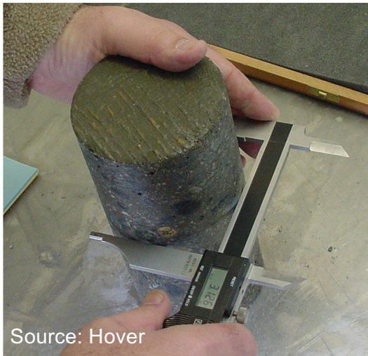
ASTM C597 Ultrasonic Pulse Velocity Source: Hover
