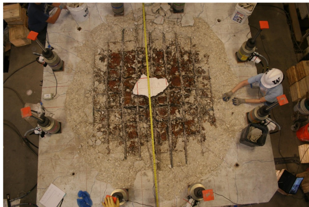
Post-test condition of slab-column connection tested, with corroded reinforcement.
