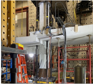
Laboratory slab-beam-column tests. (1 of 2 tests in progress)
