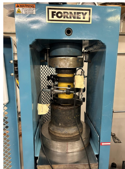
Compression strength tests of concrete cores with variable moisture content.
