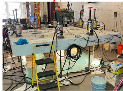
Laboratory slab-column connection test. (3 of 8 complete)
