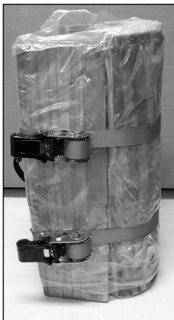
Figure 3-14. A Tightly Wrapped Bundle with Straps Placed at 10 cm (4 in).
