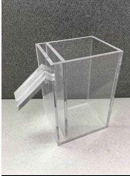
Figure 3-7(a). Example of a Displacement Vessel.
