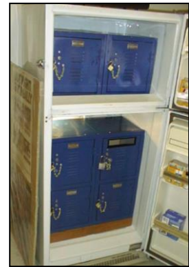
Figure III-14: Modified residential refrigerator.
