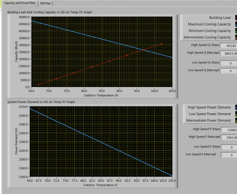
Building Load is 10% lower than the 95°F (35°C) capacity and zero at 65°F (18.3°C)
