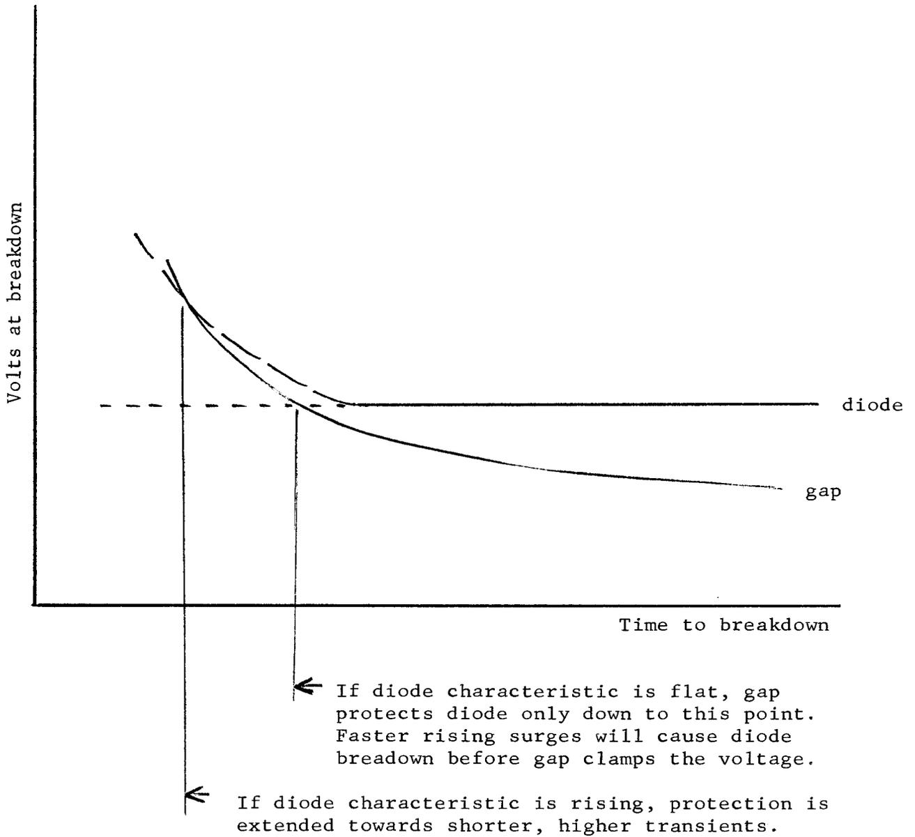
Coordination of gap and diode characteristics
