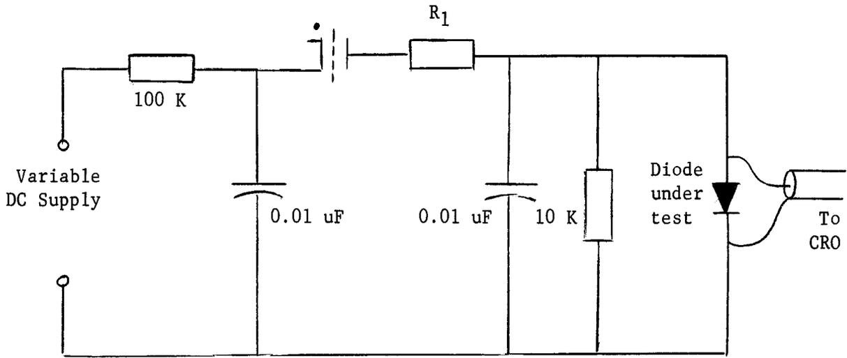
$R_1$  adjusted from 25 ohms to 2,000 ohms to change time to crest (and thus rate of rise) of the impulse.
