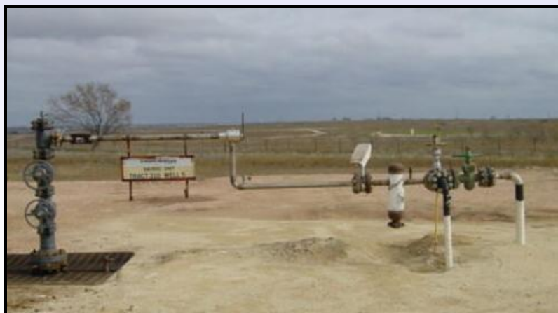
Injector well with both CO 2 and water for WAG EOR
